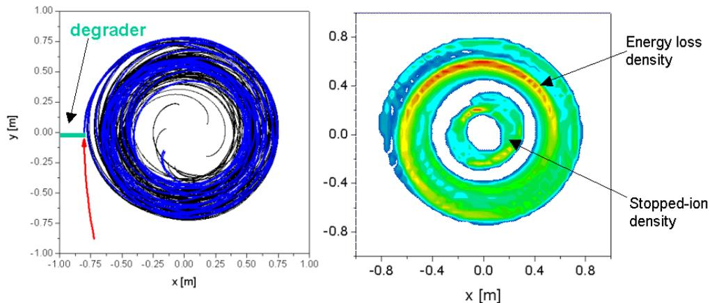
Figure 1: Sample trajectories of 100 MeV/u <sup>78</sup>Br ions in a 2-T cyclotron gas stopper with 10 mbar He pressure (left). Energy loss density and stopped-ion distribution (right).
