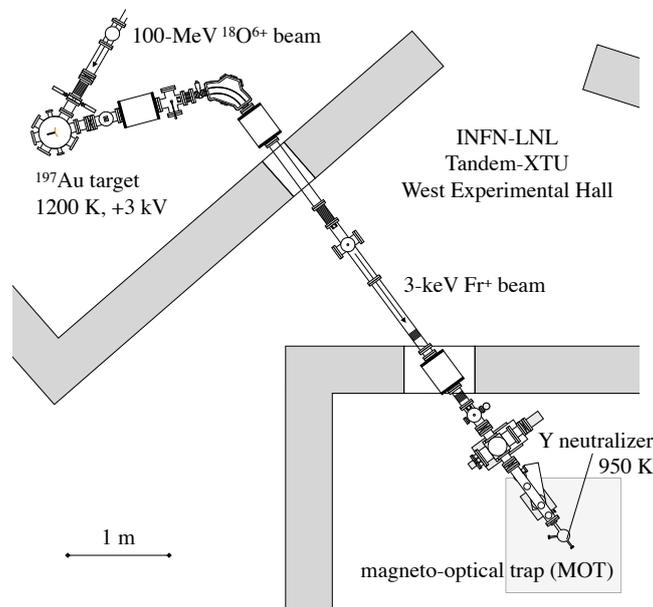
*Layout of the experimental apparatus.*
