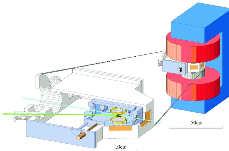
Figure 1: Overview of the polarized proton target.
