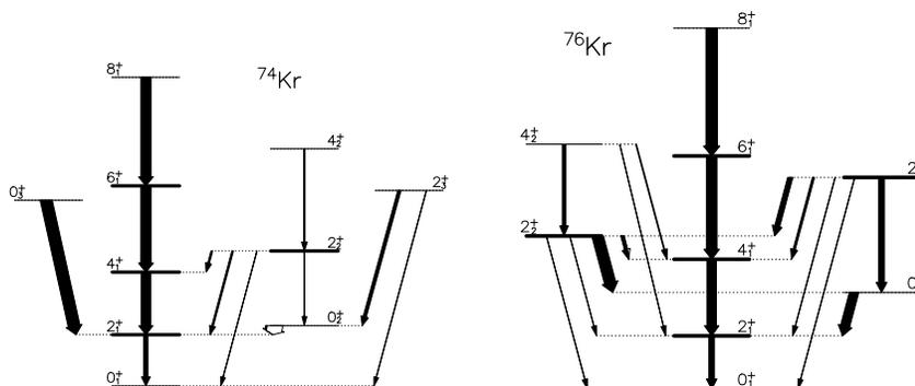
Figure 1: Partial level schemes of  $^{74}\text{Kr}$  and  $^{76}\text{Kr}$  showing all transitions for which  $B(E2)$  values were determined. The width of the arrows corresponds to the transition strengths. The states for which the static quadrupole moment was measured are shown with bold lines.
