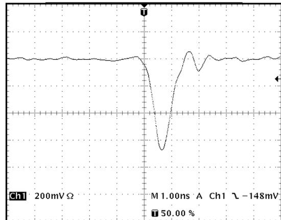
**Figure 1:** Preamplifier signal for a single-particle event. 100 MeV/u  $^{76}\text{Ge}$  ions were used to irradiate the detector.
