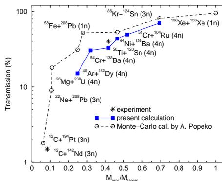
Figure 1: Transmission of the velocity filter SHIP. Squares represent the results of the present simulations, stars experimental values and circles refer to previous calculations performed by A. Popeko[5].
